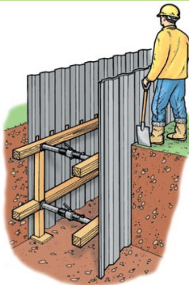
Trench sheets with timber walings, screw props, punchions and sole plates
